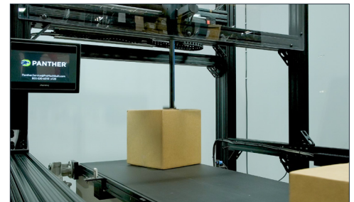
Adaptive labeling technology automatically adapts to changing product heights to keep production moving without interruption.
